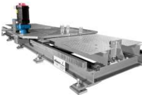
Robot Tracks, Hardened guides, Travel 2 m/s, repeatability +/-0.1mm, Floor leveling/adjustment feature.
