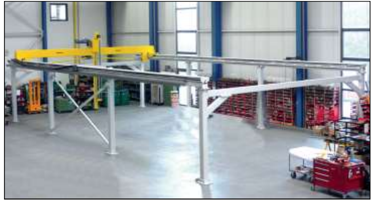
Single Bridge Gantry with X, Y and Z-Axis Control
