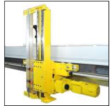
Dimensions horizontal axis, Type PLE-100 ZS-H, rack and pinion drive for load capacity up to 100 kg, speed to 5 meter per second and repeatability from 0.5mm.
