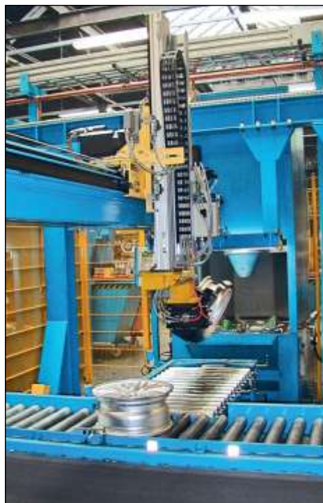
Vertical Telescoping , work piece handling, load 200kg.
